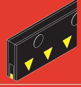
The construction of the blades features a core of carbide inlays embedded in rubber, keeping the blades more elastic and flexible. This greatly reduces vibration and noise and helps keep the blades from jumping or "chattering."
